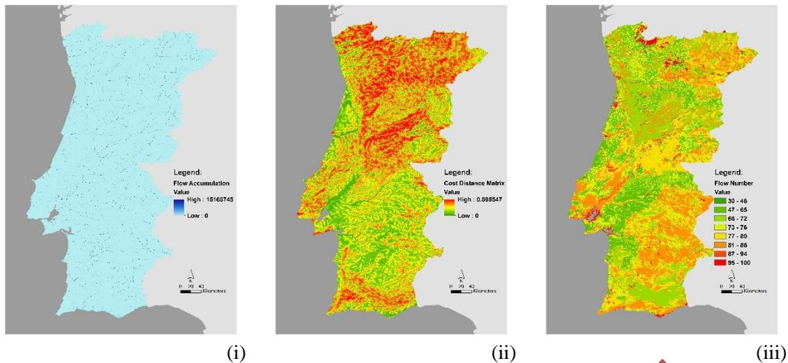
**Figure 3 – Maps of the original variables used in the flood susceptibility index: i) Flow Accumulation ; ii) Cost Distance Matrix; iii) Flow Number**
