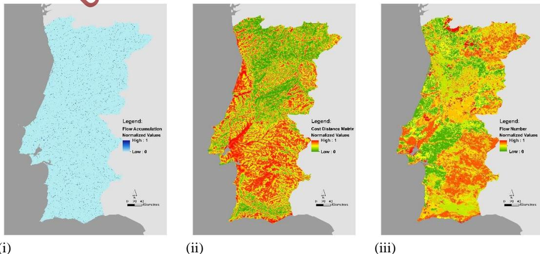
**Figure 5 - Normalized variables used in the flood susceptibility index: i) Flow Accumulation ; ii) Cost Distance Matrix; iii) Flow Number.**
