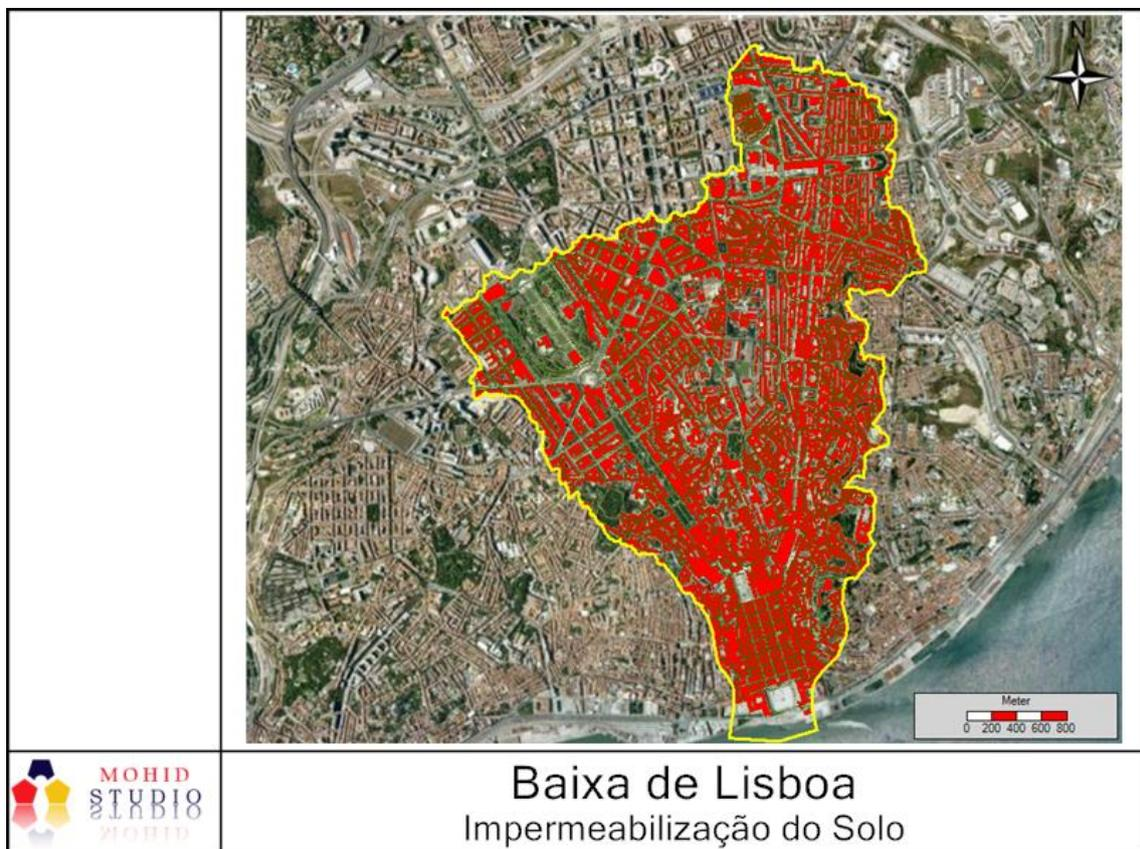
Figure 20: Estimated soil impermeability (obtained from buildings and streets)
