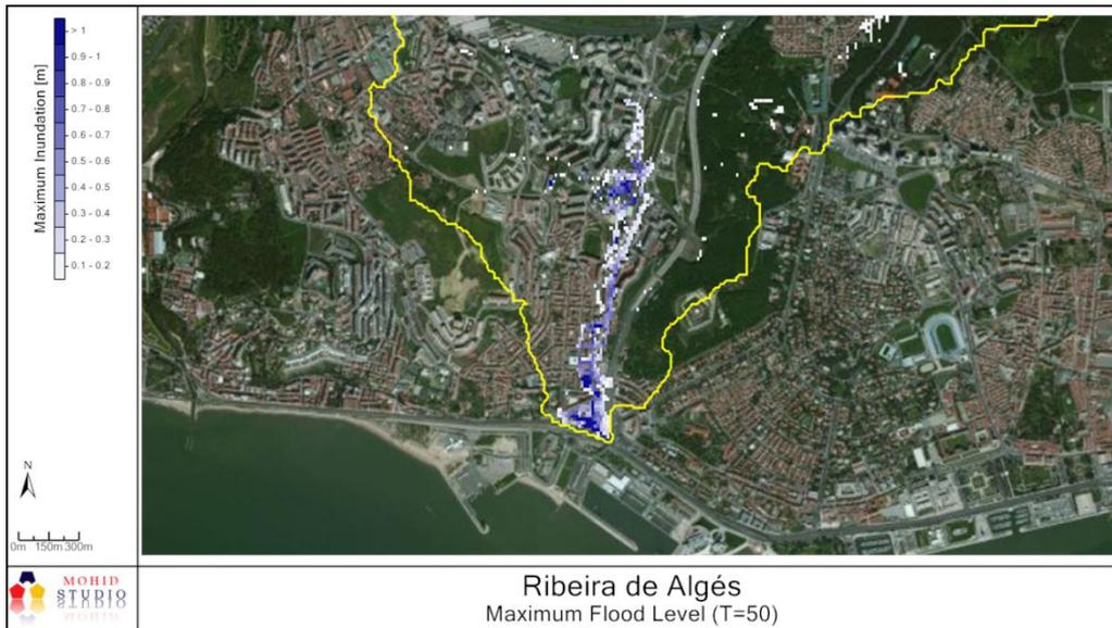
**Figure 14: Maximum expected inundation depth (T=50 years)**
