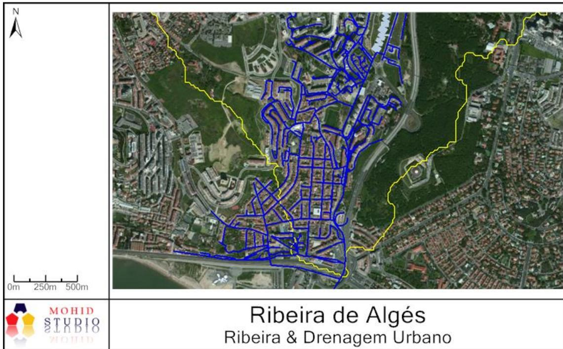
**Figure 9: Storm water drainage system simulated by the SWMM model**
