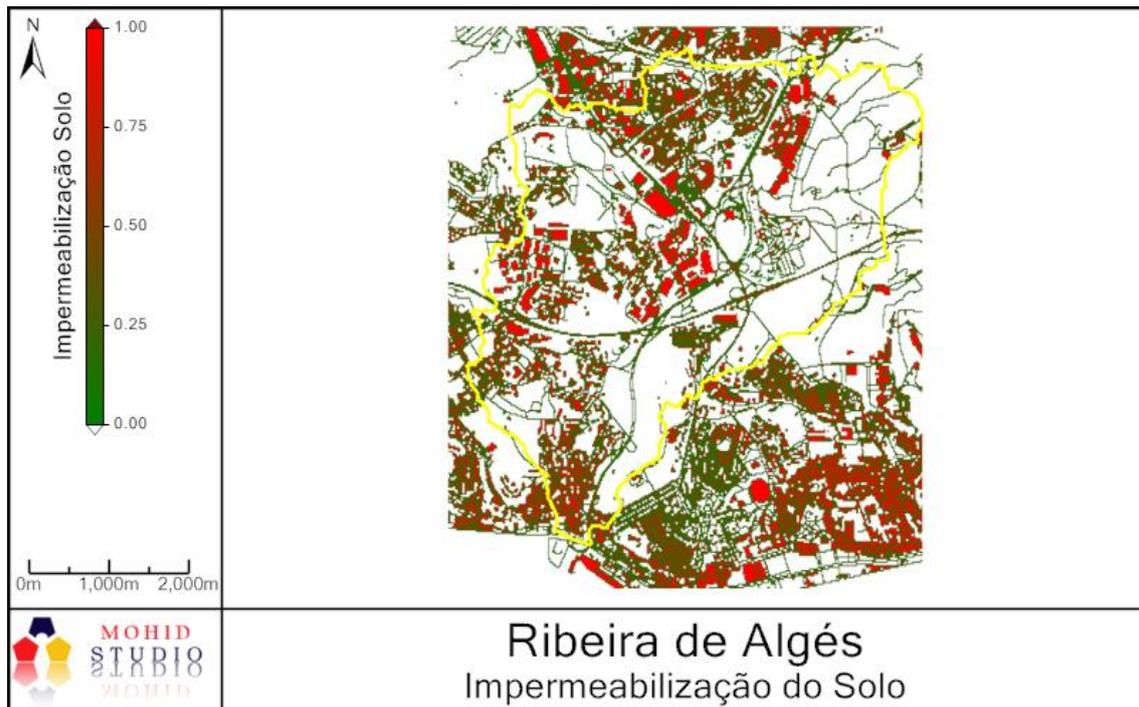
Figure 11: Estimated soil impermeability (obtained from buildings and streets)
