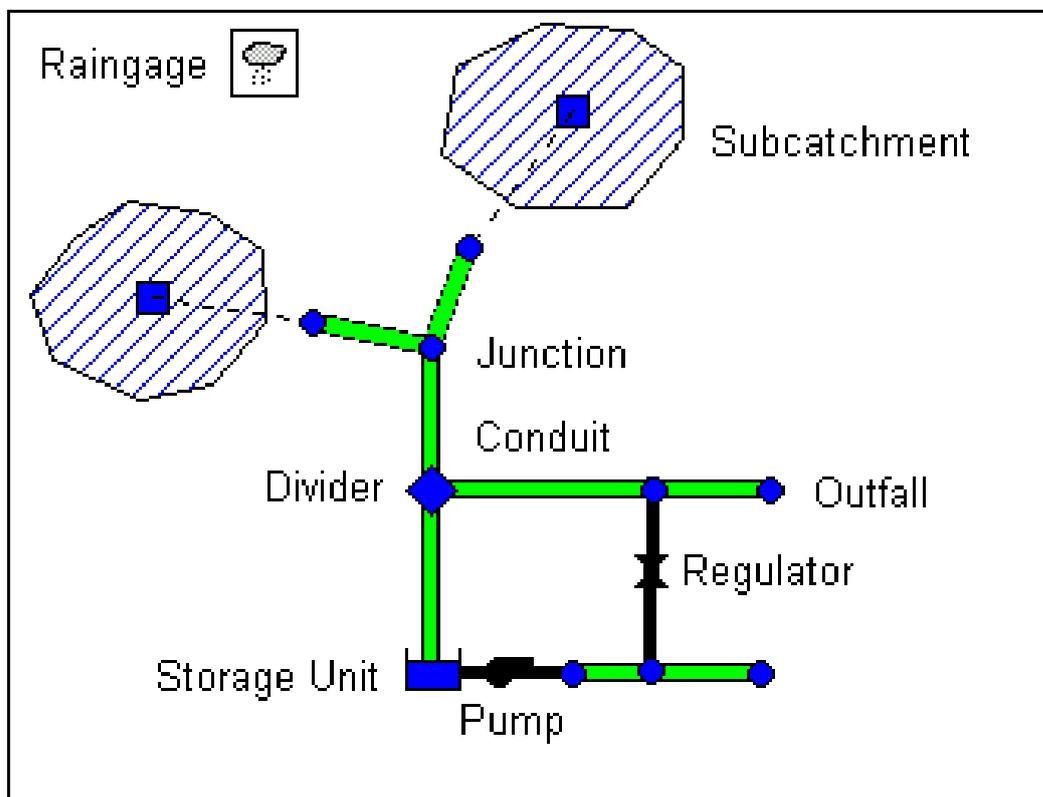
**Figure 4: Schematic representation of the SWMM model**
