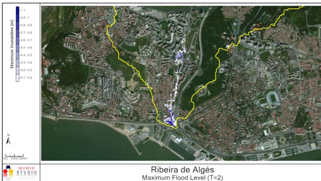
Figure 13: Maximum expected inundation depth (T=2 years)
