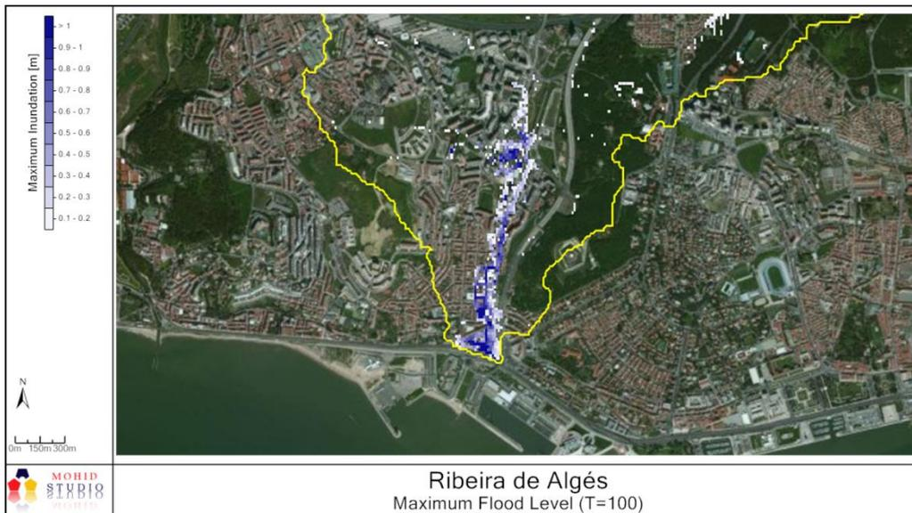
**Figure 15: Maximum expected inundation depth (T=100 years)**
